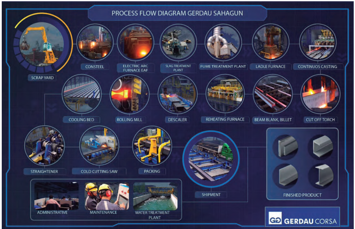
Figure. 1. Flow diagram of hot rolled structural shapes manufactured from steel scrap.
